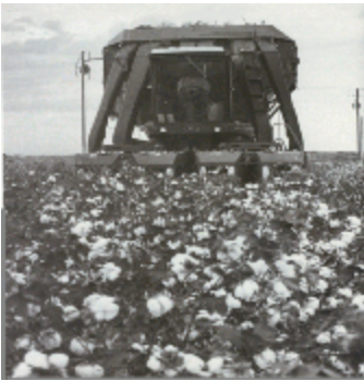
Harvesting Cotton with a Stripper
